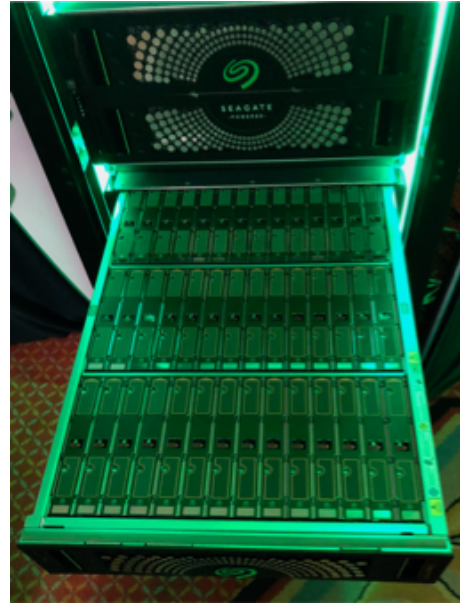
Seagate Cloud Scale Storage Array (1 PB in 5U)
