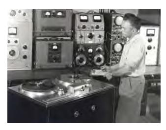
Ampex Model 200 magnetic tape recorder (1947)
