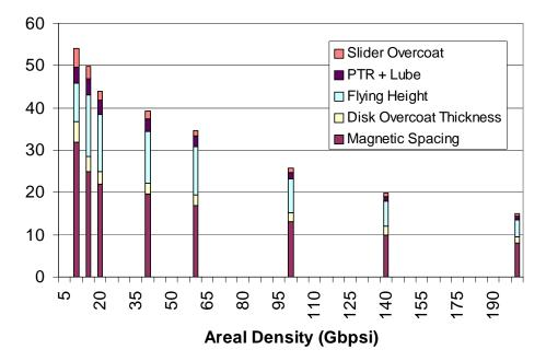
A lower flying height creates greater demands on disk cleanliness and topography in order to avoid errors in reading back the information on the disk drive. In addition higher recording densities creates greater sensitivity to smaller disk defects.
