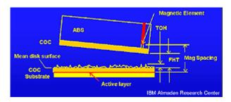
Figure 3. Magnetic Spacing Component Roadmap
