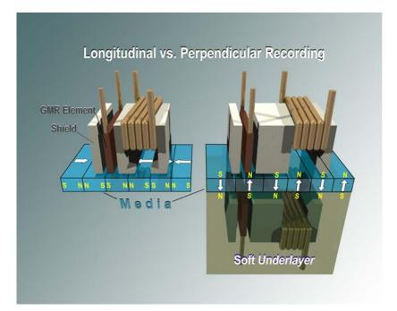
Perpendicular recording has its own special issues however. In order to maintain a consistent write field on the media the spacing between the head and the disk must have a lower flying height and tighter spacing loss tolerance and the write head poles require special shaping in order to prevent write fields going through the media soft magnetic layer to weaken and even overwrite adjacent track data.
